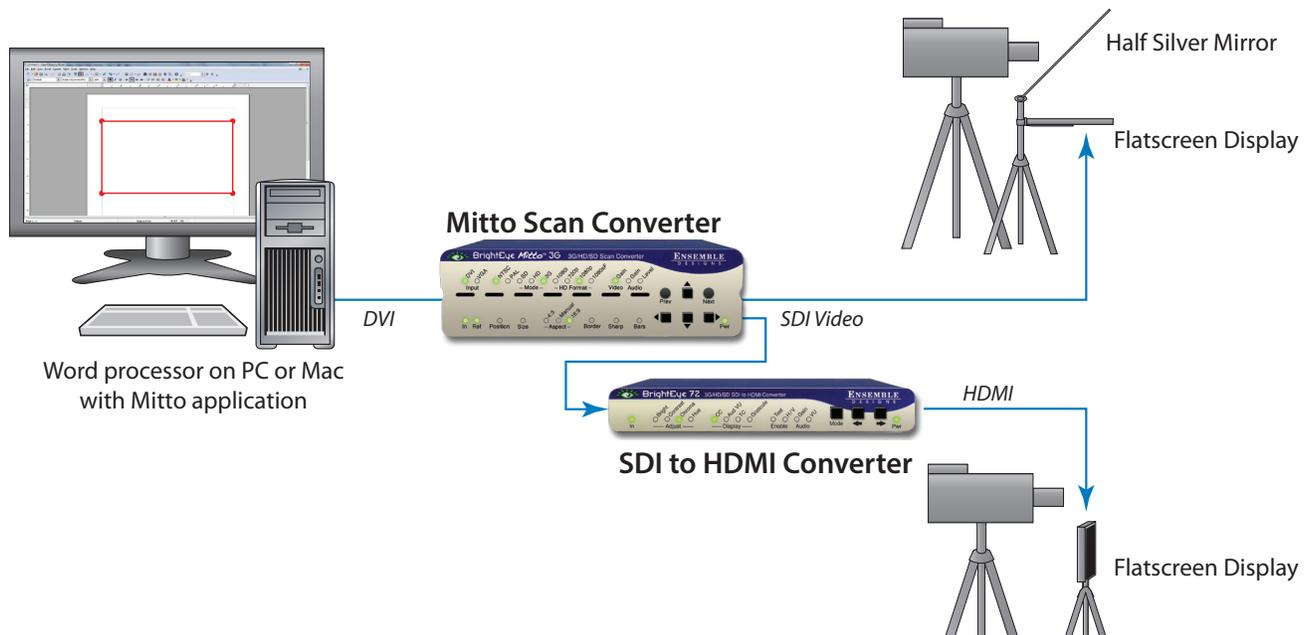
The BrightEye Mitto scan converter can be used with applications such as Microsoft Word or PowerPoint™ to provide an effective teleprompting solution without breaking the bank.
